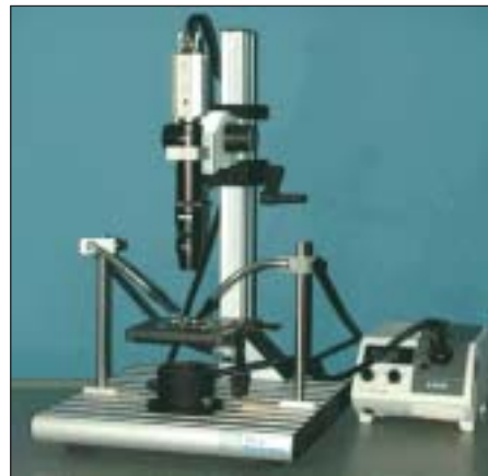
Manual X, Y stage adapted for a Navitar ® zoom on a Tech Systèmes ® bench.
