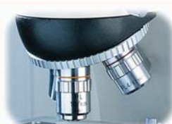
Reversed nosepiece with plan achromatic objectives
