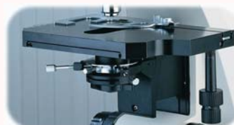
Smooth, coaxial control mechanical stage with slide holder
