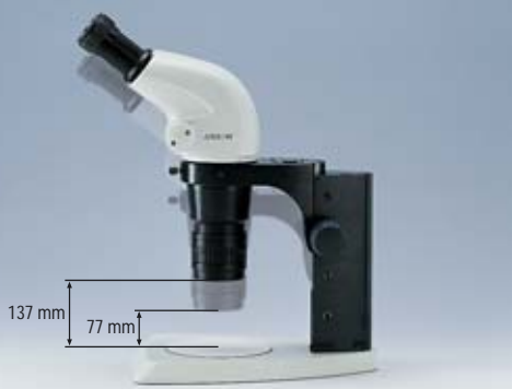
Ergonomic objective 0.6x – 0.75x on Leica S6 E, working distances 77mm to 137mm
